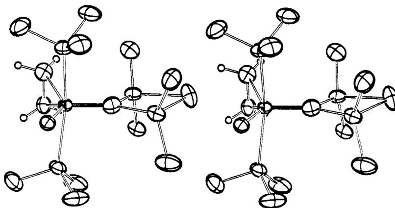
**Figure 3.** Stereoscopic view of the  $W(CAl_2Me_4Cl)(CH_3)(PMe_3)_2(\eta^2-C_2H_4)$  molecule. All hydrogen atoms except the ethylenic hydrogen atoms are omitted for clarity. The view in this figure is related to that in Figure 2 by a rotation of approximately  $95^\circ$  about the  $W-C(3)$  axis (ORTEP-II diagram; 30% ellipsoids).
